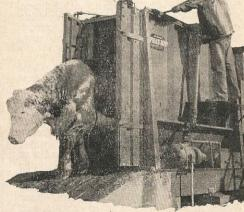
Two offset rows of teeth rake off the scabs, while 3 powerful jets (15 GPM) pour insecticide into the grub holes for sure-fire grub control. Light . . . all aluminum with instant cutoff.
